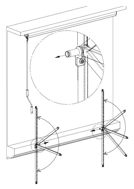
Adjusting the arm degree in right position and close the awning and ensure the fabric tight.
