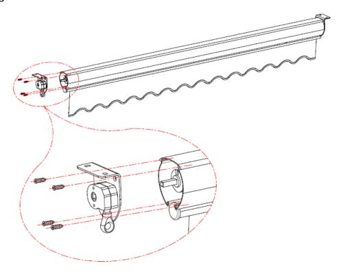
Loosen the screws as drawing B and take out the the gearbox as drawing C; Rotating the bracket 90 degree as drawing D and finding the right holes as drawing E and fastening the screws as drawing F.
