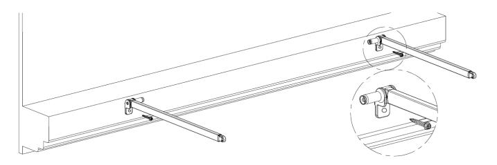
Retracting out the fabric fully, then hang the arm hook part into front bar hook and move front bar hook until the arm being horizontal and fasten the screws of hook.
