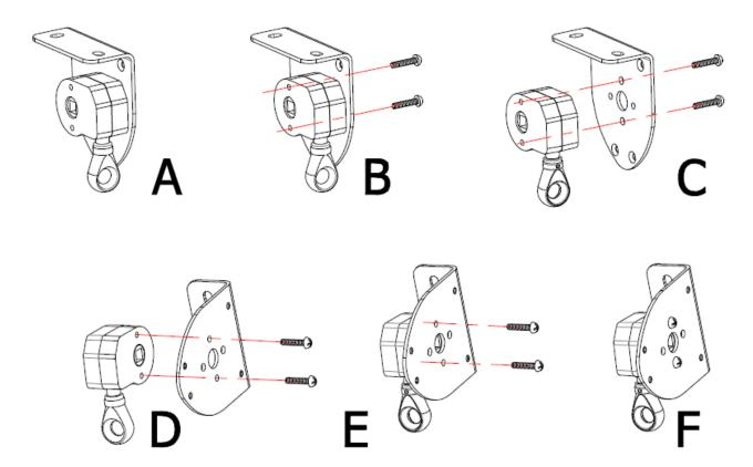
3. Fasten the screws of the brackets assembled with gear box to the awning cassette as below drawing and insert the round end cap to another bracket hole and ensure the square end cap to bracket.
